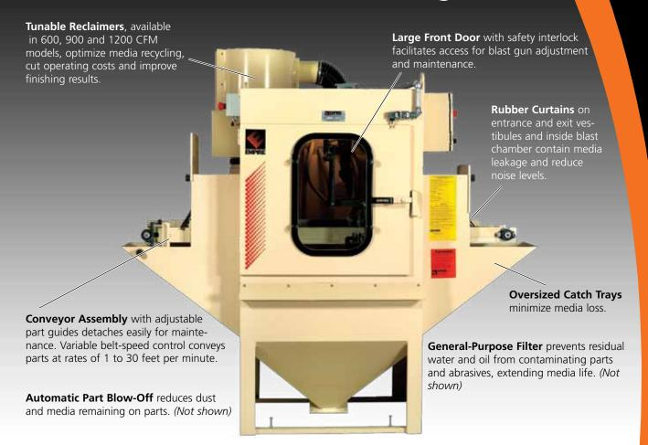
Based on Empire's field-proven Pro-Finish® technology, the IL-885 incorporates a rugged conveyor assembly driving a 9-inch-wide by 72-inch-long belt. Variable speed controls and adjustable parts guides provide the versatility to deburr, clean, profile and finish parts of many different shapes and sizes ranging from tubular to flat; if two sides of a workpiece require blasting, the piece can be reloaded for a second pass.
